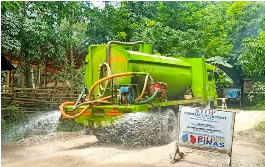
4 Clean air. A water truck sprays roads as part of TVIRD's dust suppression activities during the dry season.
